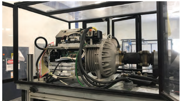
Figure 2. Danfoss Turbocor compressors from Pennsylvania site in Tallahassee testing facility.
